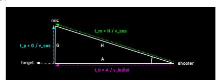
If we look at the triangle from the shooter's perspective, the projectile travels at projectile velocity  $(v_b)$  along the trajectory (A) and generates the crack at the moment of closest approach to the microphone. This crack then travels along the vertical line (G) at the speed of sound. G and A represent the opposite and adjacent sides in the right-angled triangle.
