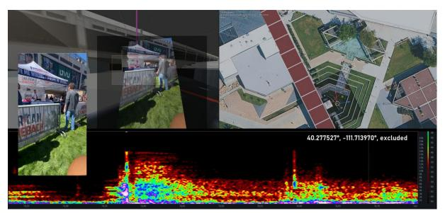
This camera contains a clearly recognizable audio pattern. However, the measurable times differ so greatly from neighboring cameras that it is possible that the sample frequency was also changed during post-processing, e.g., frame rate conversion.
