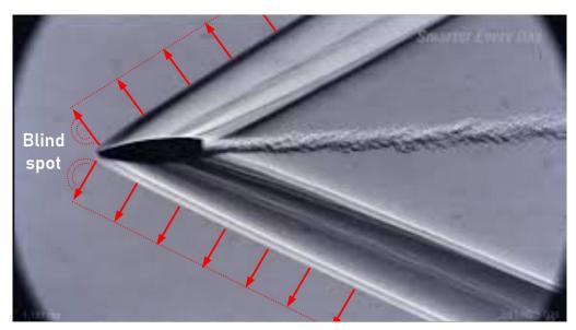
If the trajectory ends by hitting a target, a crack wave is no longer generated. This means that a dead zone is created behind the target, in which no crack can be heard. Near the edges of the ending wave, there may still be decaying effects due to diffraction and the wave fading out, but in general, no crack is to be expected in the dead zone.
