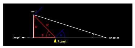
The easiest way to do this is to reduce the Mach cone model to the original right-angled model by "correcting" the measured  $\Delta t$  for the hypothetical case in which the crack would actually have to take the detour via the right angle. This means we calculate the time difference between the two paths and correct the measured "shortcut" via H'. The difference is as follows:
